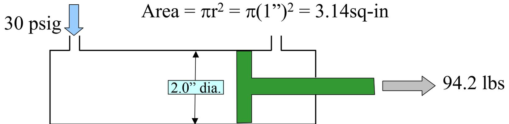
$$\text{Force} = 30 \text{ psi} \times 3.14 \text{ sq-in} = 94.2 \text{ lbs}$$
