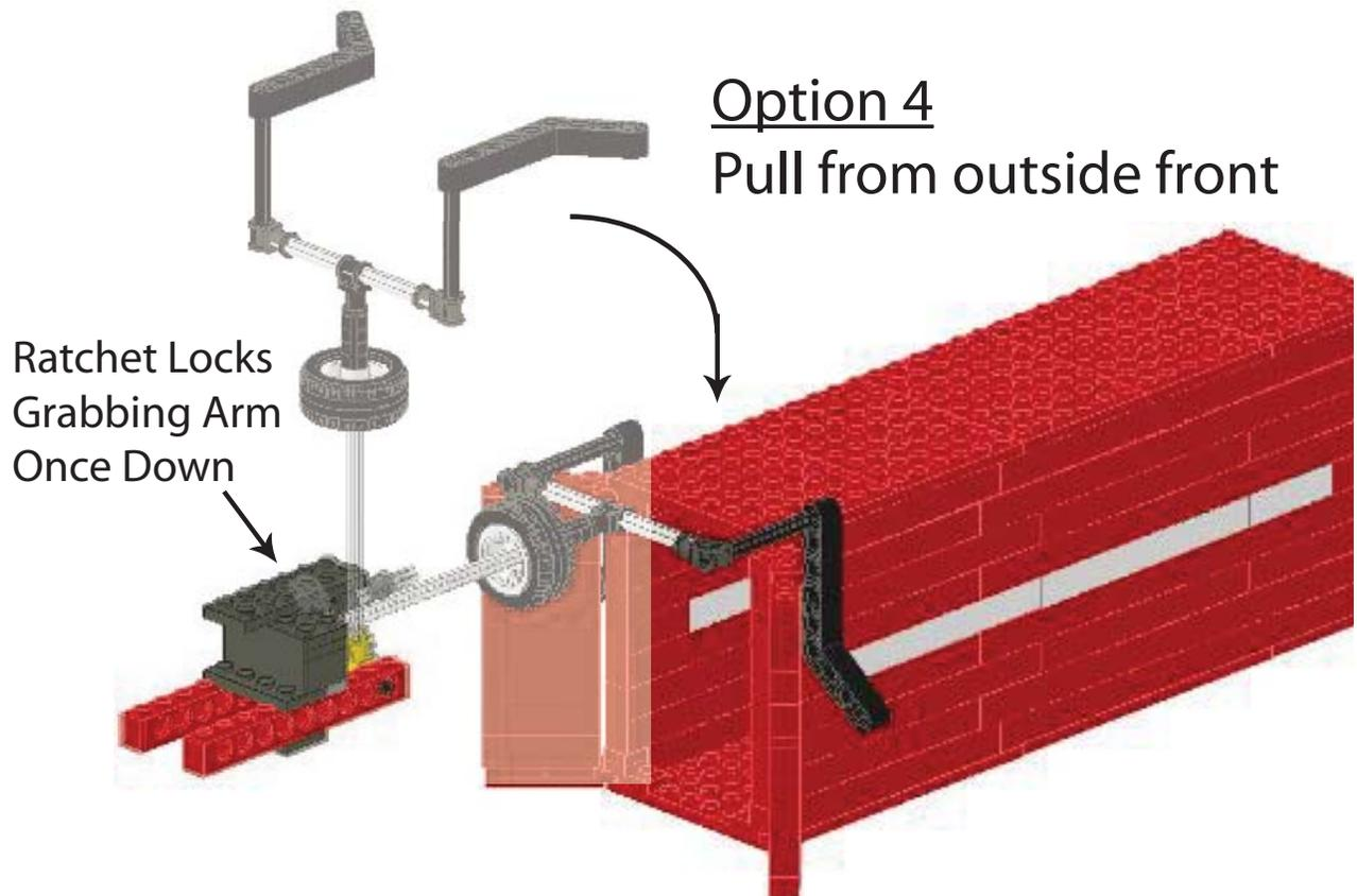
Here is the closeup of the ratchet with some pieces removed to show how the mechanism worked. As the large grabbing arm fell, it would drag on the bushing noted below which acted as a pawl to the 24 tooth ratchet gear.
