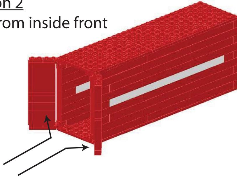
The third option that worked and was most reliable was to have a mechanism to grab it from the front. Again the weight of the container is an issue so there was a tendency for the forked grabbing arms to slip up and off. However, a pawl and ratchet built into the drop down mechanism overcame this issue.
